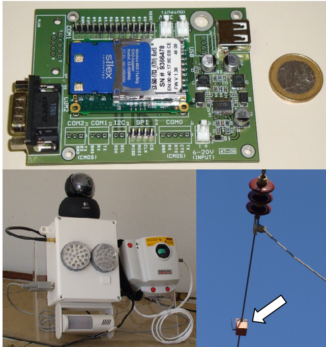
Figure 2. Top: Sillex sensor with PCB; Bottom-left: Sensor with webcam, infrared camera, LED light and movement sensor; Bottom-right: Sensor hanging on a 15 KV line, harvesting energy from the line.
