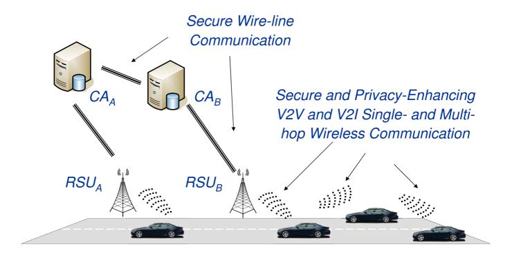
Fig. 1. Abstract View of the Secure Vehicular Communication System.
