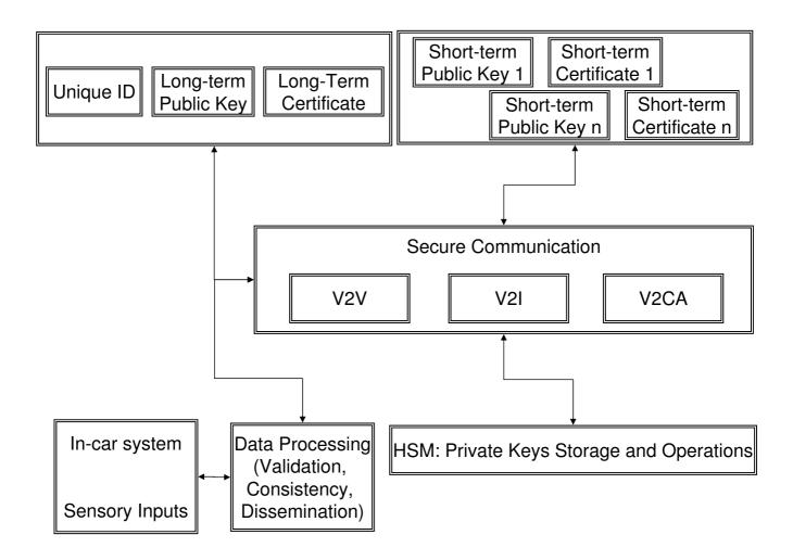
Fig. 2. Conceptual Secure VC Architecture View: Node functionality.
