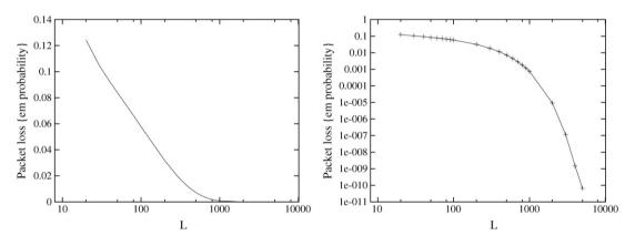
Fig. 2. Packet loss probabilities (y-axis on the linear and log scales respectively).
