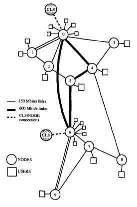
Fig. 5. Topology of the simple network used for the efficiency tests.
