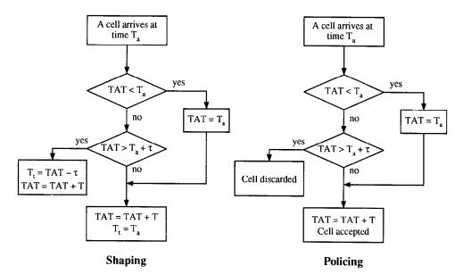
Fig. 1. Flow chart of the GCRA for shaping (left) and for policing (right).
