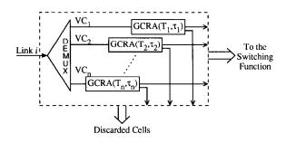
Fig. 3. Architecture for traffic policing.
