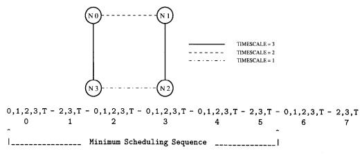
Fig. 4. Scheduling sequence for a network with different link data rates; T is the timing event.
