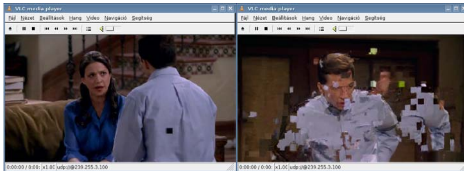
Figure 11. The result of packet loss ratio of 0.1% (left side) and 1% (right side)
