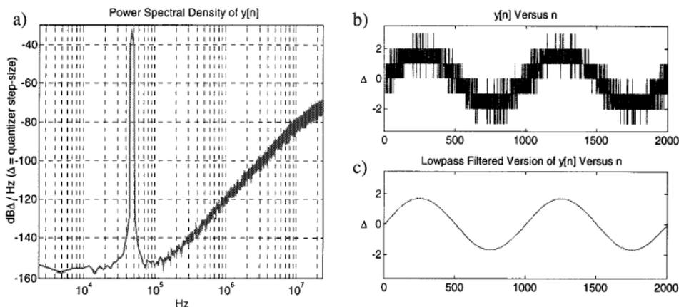
Fig. 4. (a) PSD plot of the ΔΣ modulator output in decibels, relative to the quantization step-size, per hertz. (b) Time-domain plot of the ΔΣ modulator output. (c) Time-domain plot of the ΔΣ modulator output filtered by a sharp lowpass filter with a cutoff frequency of 500 kHz.
