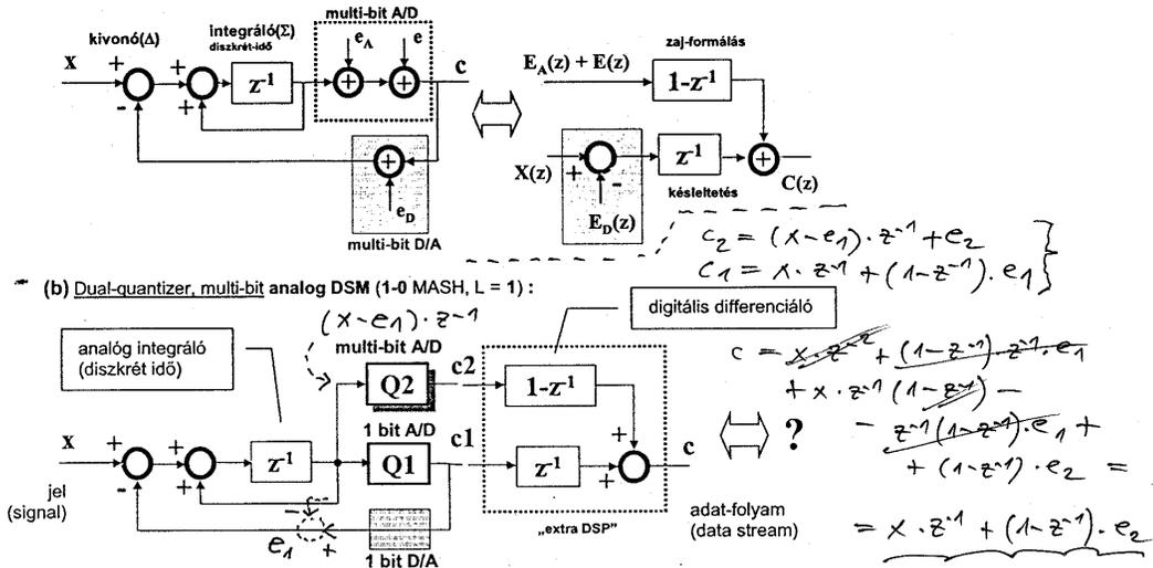
(b) Dual-quantizer, multi-bit analog DSM (1-0 MASH,  $L = 1$ ):
