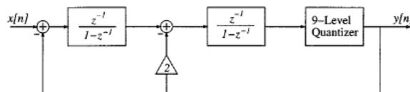
Fig. 3. Second-order ΣΔ modulator architecture.
