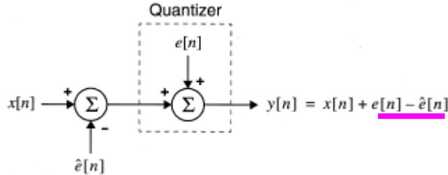
However, since the error is not known until it is made,  $e[n]$  is not known when  $\hat{e}[n]$  is needed. Therefore, some means must be found to estimate the error.
