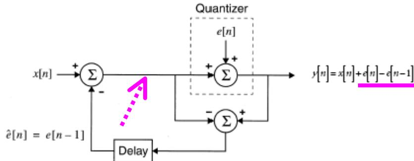
With a few straightforward steps, the system can be transformed into that of Fig below, where the delay element is now immersed in an integrator feedback loop.
