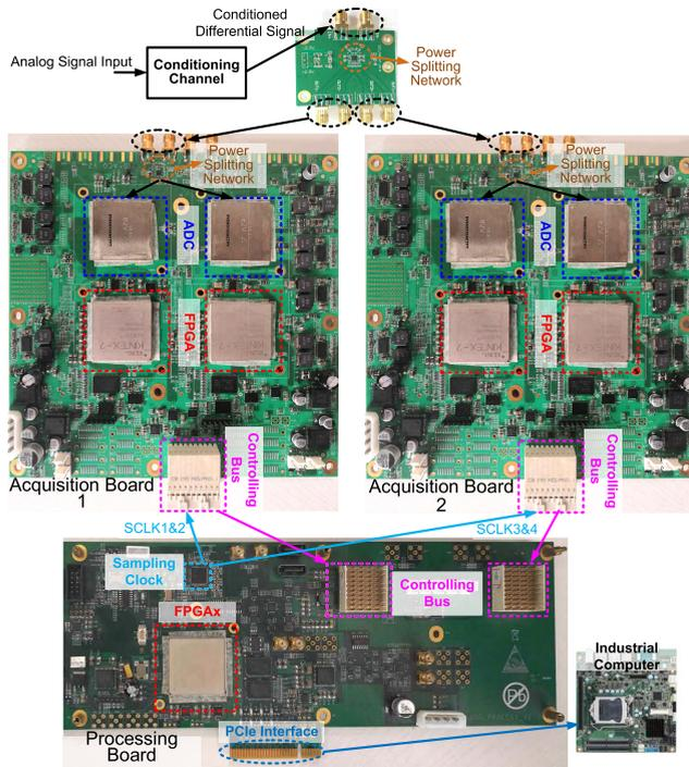
**FIGURE 10.** The material diagram of multi-resolution UF-DAQ prototype with four-channel hybrid sampling structure.
