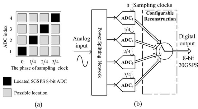
**FIGURE 7.** The time-interleaved scheme of highest sampling rate with four 5GSPS ADCs: (a) 20GSPS 8-bit arrangement topology, (b) its system diagram.
