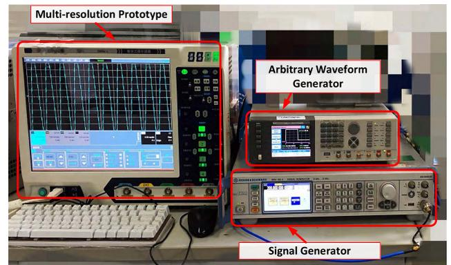
**FIGURE 11.** The test platform of multi-resolution UF-DAQ prototype.
