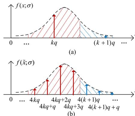
**FIGURE 3.** A PDF instance of output signal in (a) single channel and (b) 4-channel TSADC system.
