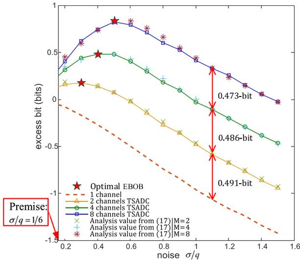
FIGURE 5. Numerical result of EBOB in the theory and simulation based on TSADC structure.
