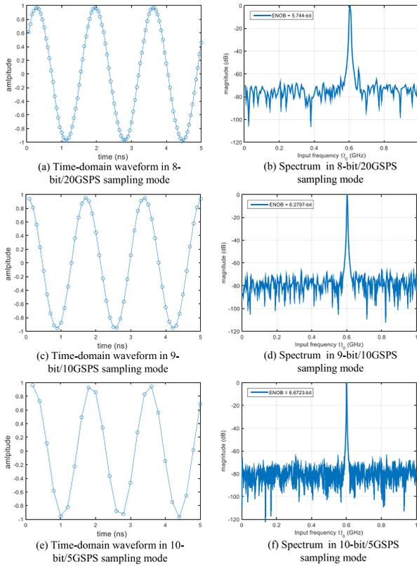
**FIGURE 14.** Time- and frequency-domain results of the prototype at different sampling modes with 600MHz sinusoidal signal input.
