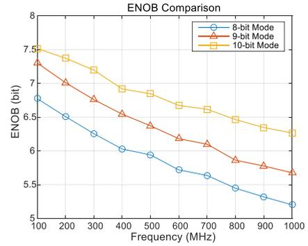
**FIGURE 15.** ENOB curves with different input frequencies and in different resolution modes.
