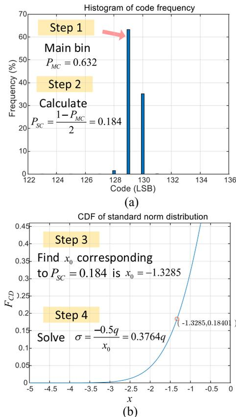
**FIGURE 12.** Experimental results of noise evaluation: (a) the histogram of digital code frequency and the instance of step 1&2; (b) the curve of CDF of standard norm-distribution and the instance of solving the RMS value of thermal noise at the step 3&4.
