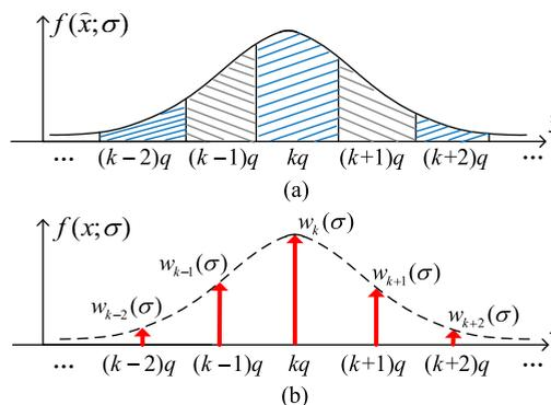
**FIGURE 2.** PDFs of quantizer (a) input and (b) output in the case of DC signal with thermal noise.
