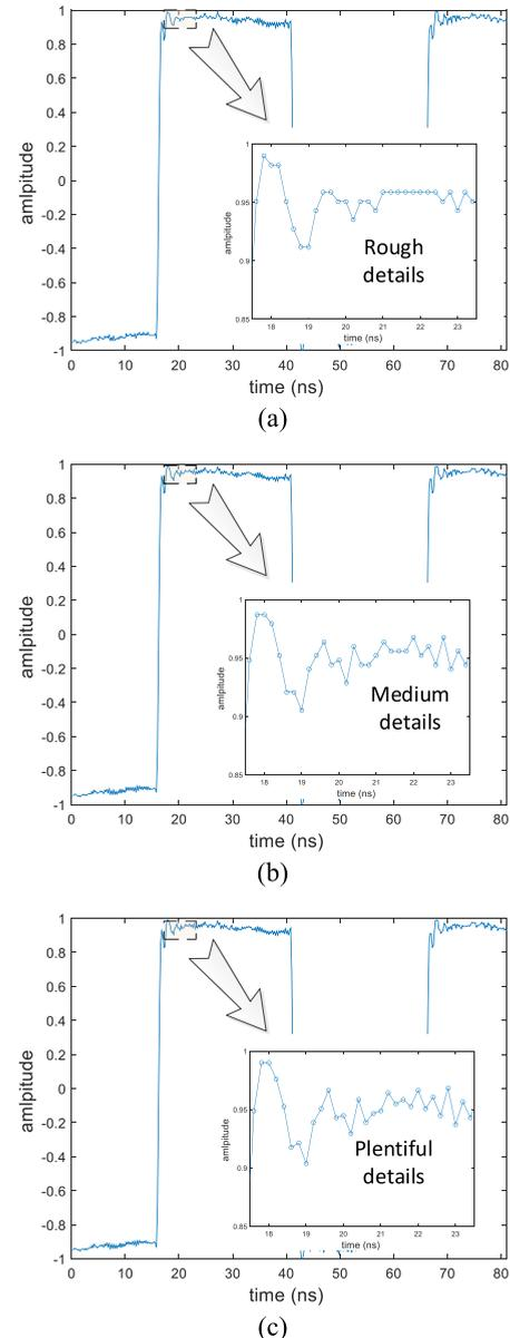
**FIGURE 13.** Time-domain waveforms of 20MHz square signal by (a) 8-bit (b) 9-bit and (c)10-bit sampling modes. The inside window is the zoomed view of waveform.
