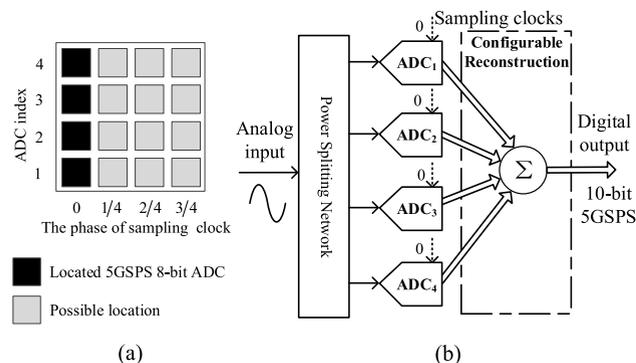
**FIGURE 8.** The time-synchronized scheme of highest resolution with four 5GSPS ADCs: (a) 5GSPS 10-bit deployment topology, (b) its system diagram.
