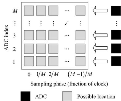
FIGURE 6. The general arrangement diagram of multi-component locations for multi-resolution UF-DAQ applications.
