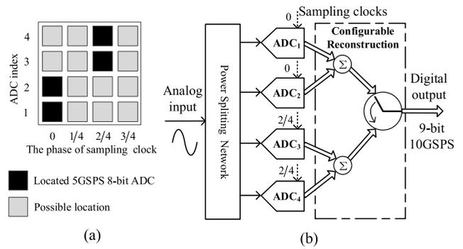
**FIGURE 9.** The novel hybrid scheme of trade-off performance with four 5GSPS ADCs: (a) 10GSPS 9-bit deployment topology, (b) its system scheme.
