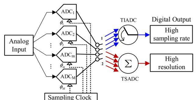
**FIGURE 1.** The structure of parallel ADC array.
