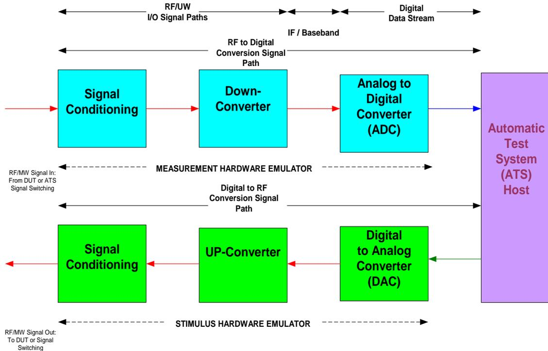
Fig. 1 Synthetic Instrument Based ATS: Notional Block Diagram
