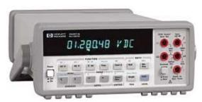
The **reading** error term is from inaccuracies in amplifier gains, divider ratios or internal reference voltages. The **range** error term is from inaccuracies in amplifier offsets, leakage current effects and thermocouple effects. Total measurement error is the sum of the readings and range errors.
