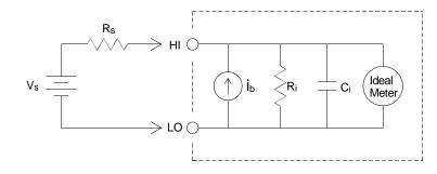
$i_b$  = multimeter bias current  $R_s$  = DUT source resistance  $C_i$  = multimeter input capacitance For DCV ranges: 0.1V, 1V, 10V:  $C_i$  < 700 pF 100V, 1000V:  $C_i$  < 50 pF For all ACV ranges: < 50 pF
