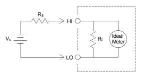
$V_s$  = ideal DUT voltage  $R_s$  = DUT source resistance  $R_i$  = multimeter input resistance ( 10 M $\Omega$  or >10 G $\Omega$  )
