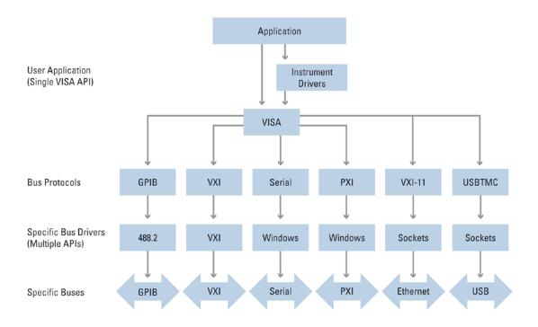
VISA changed instrument control and the test industry by abstracting the differences between buses, incorporating bus protocols, and providing a unified *API* (application programming interface) to communicate to test equipment—regardless of communication bus.
