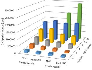
FIGURE 4. Comparison of NSD and Knot DNS for DNS64 benchmarking. (The N node result of Knot DNS at 16 cores are limited by Tester performance.)
