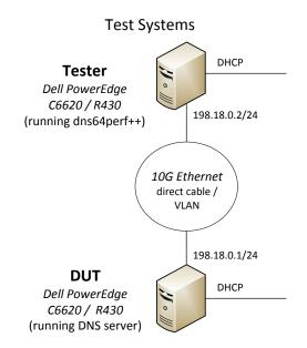
FIGURE 2. Measurement setup for all types of measurements.
