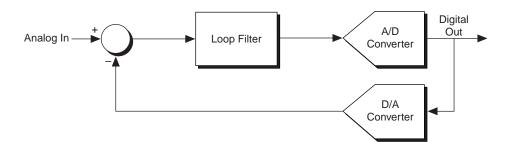
Figure 3. Block Diagram for a Multibit Delta-Sigma Converter
