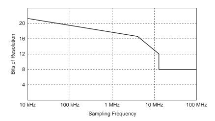
Figure 2. Resolution as a Function of Sampling Frequency for the National Instruments Flexible Resolution ADC Module
