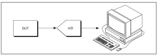
Figure 1. The Concept Behind Virtual Instrumentation
