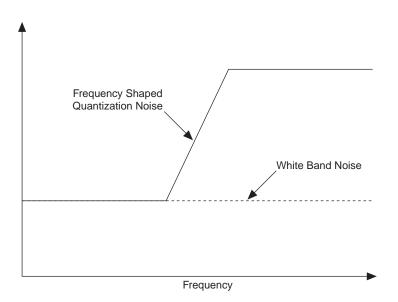
Figure 7. Broadband Noise Applied to the Noise-Shaped Output
