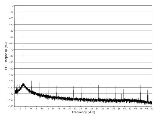
Figure 10. An FFT Plot of a 3 kHz Sine Wave 0 dB re Full Scale Measured with a Sampling Rate of 100 kHz
