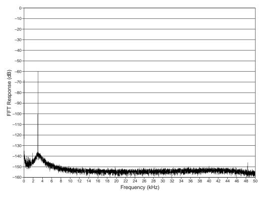
Figure 11. An FFT Plot of a 3 kHz Sine Wave at -60 dB re Full Scale Measured at a Sampling Rate of 100 kHz
