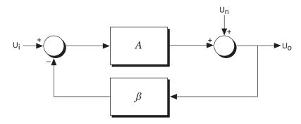
Figure 4. Block Diagram of a Servo Loop
