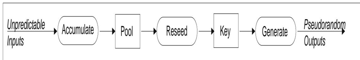
Fig. 1. Generic block diagram of Yarrow
