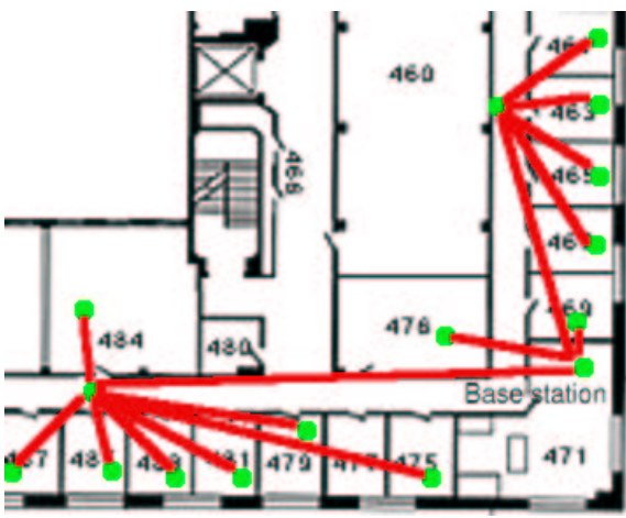
Figure 1: Communication organization within a sensor network. All messages are either destined for the base station or originate at the base station. The routes are discovered so that the number of hops is minimized and the reliability of each connection is maximized.
