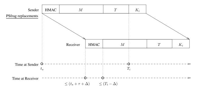
Figure 2: Timing of a packet in transmission using TIK
