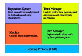
Figure 4: CONFIDANT Components in a Node (Cooperation of nodes, *S. Buchegger and J.-Y. Le Boudec*)
