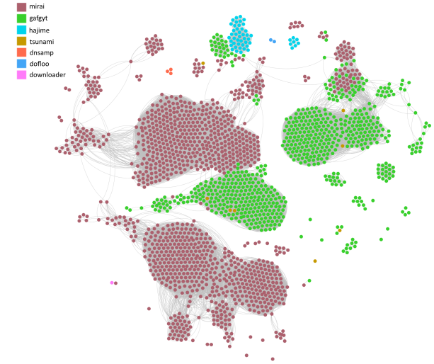
Fig. 7. Similarity graph of 2000 randomly chosen MIPS malware samples with TLSH difference threshold 40
