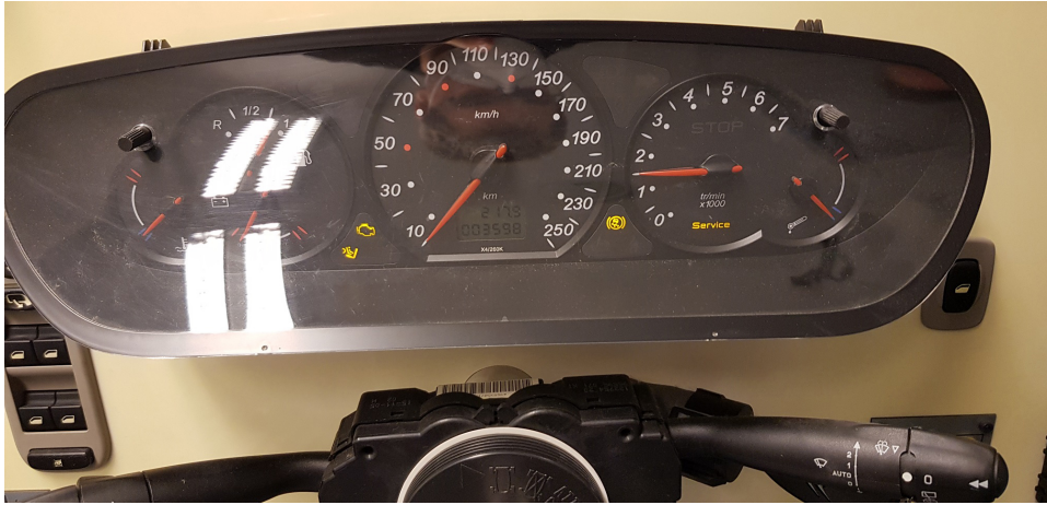
Figure 9: The attack of the tachometer displays different rpm than the real one.
