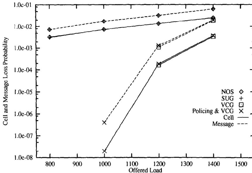
Fig. 7. Cell and message loss probabilities versus the network load, without shaping, with the SUG and VCG shaping policies, and when policing is adopted with the VCG policy.
