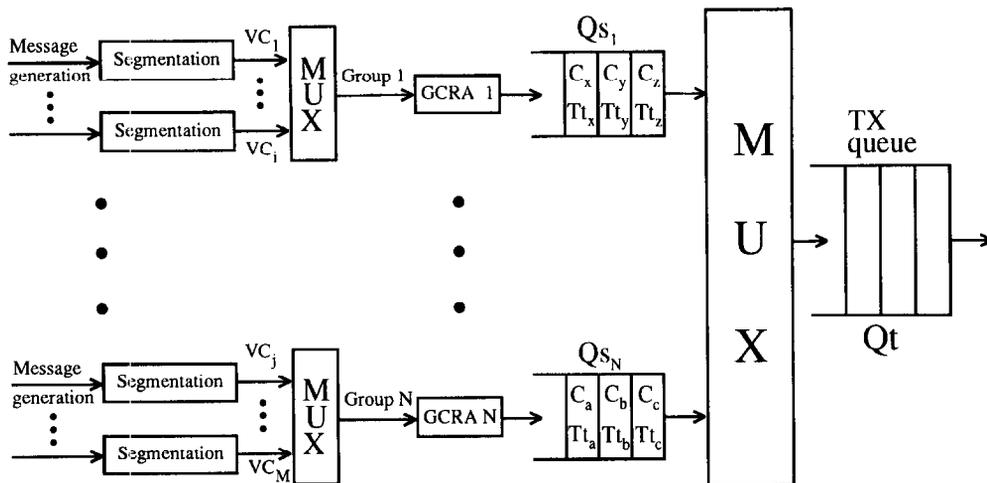
Fig. 2. Architecture for traffic shaping.
