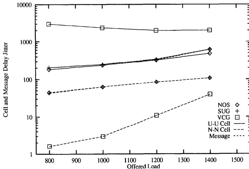
Fig. 8. Average of the user to user cell and message delay jitters and of the cell delay jitter inside the network, versus the network load without shaping and for the two grouping policies considered.
