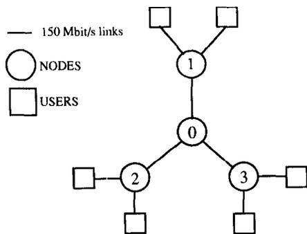
Fig. 5. Topology of the simple network used for the efficiency tests.
