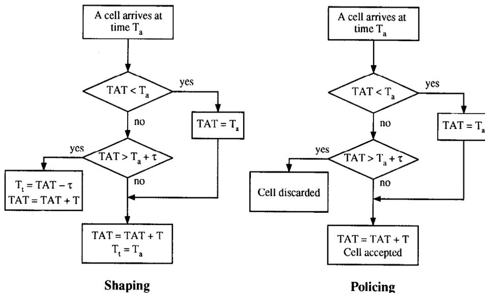
Fig. 1. Flow chart of the GCRA for shaping (left) and for policing (right).
