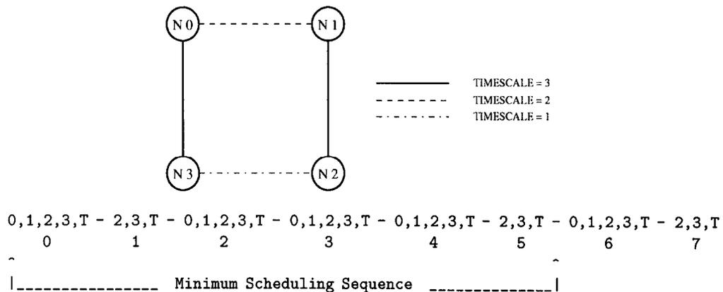
Fig. 4. Scheduling sequence for a network with different link data rates; T is the timing event.
