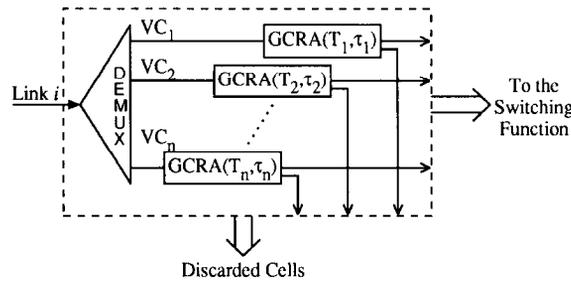
Fig. 3. Architecture for traffic policing.
