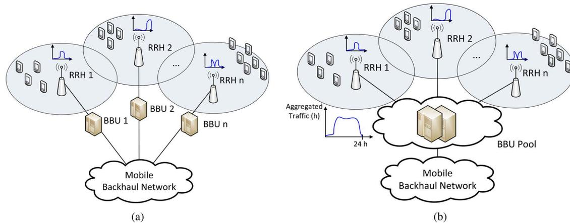
Fig. 2. Statistical multiplexing gain in C-RAN architecture for mobile networks. (a) RAN with RRH. (b) C-RAN.
