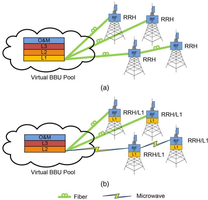
Fig. 9. C-RAN architecture can be either fully or partially centralized depending on L1 baseband processing module location. (a) C-RAN: fully centralized solution. (b) C-RAN: partially centralized solution.
