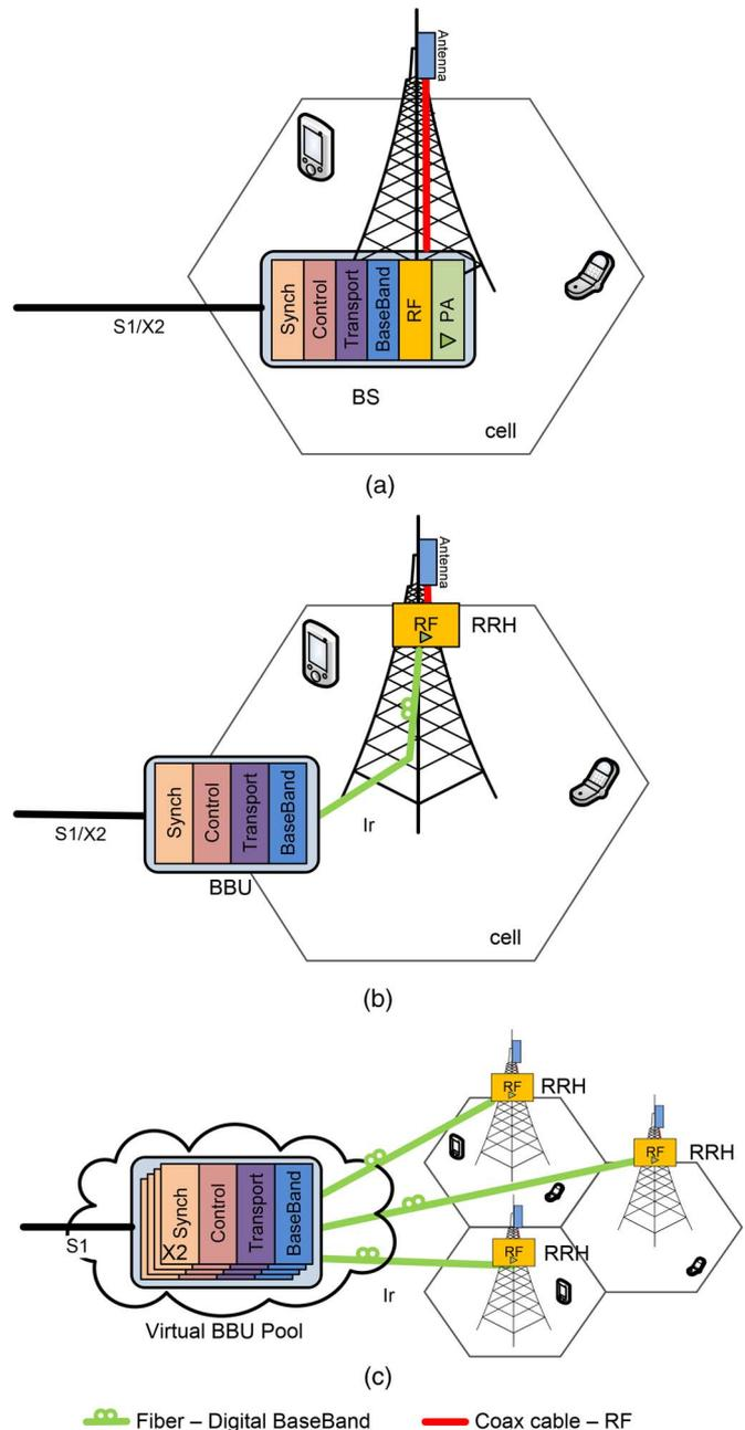
Fig. 4. Base station architecture evolution. (a) Traditional macro base station. (b) Base station with RRH. (c) C-RAN with RRHs.
