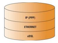
In some cases, advanced functionality ranging from local PPP and RFC1483 session termination (B-RAS offload capability) to full IP routing, AAA, security, 802.1p prioritization and DiffServ QoS is incorporated into Ethernet DSLAMs, resulting in truly IP-enabled IP-DSLAMs.
