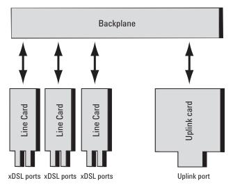
From the traffic processing perspective, two distinct architecture models have emerged – centralized and distributed.
