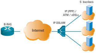
While already using Ethernet or Gigabit Ethernet uplinks, IP-DSLAMs still typically use ATM on the local loop as an intermediate layer between Ethernet and DSL – mostly for reasons of compatibility with existing xDSL modems.
