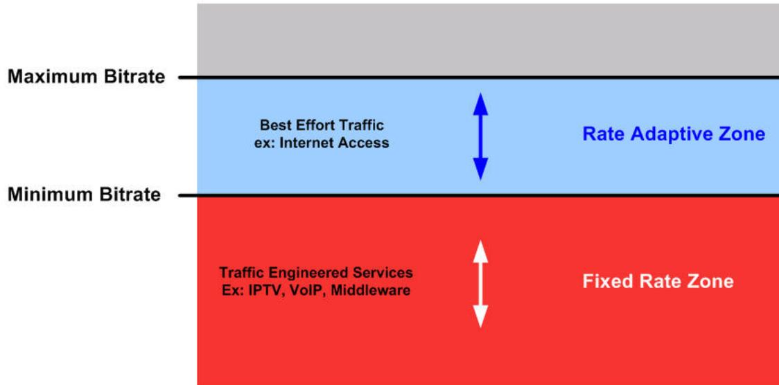
**Figure 1 - Concept of Rate-Adaptive DSL Comprising Two Components**
