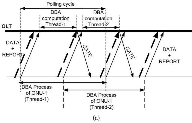
Fig. 6. Increasing the number of polling threads increases the overlapping probability of the DBA threads in a. EPON and b. GPON [44].
