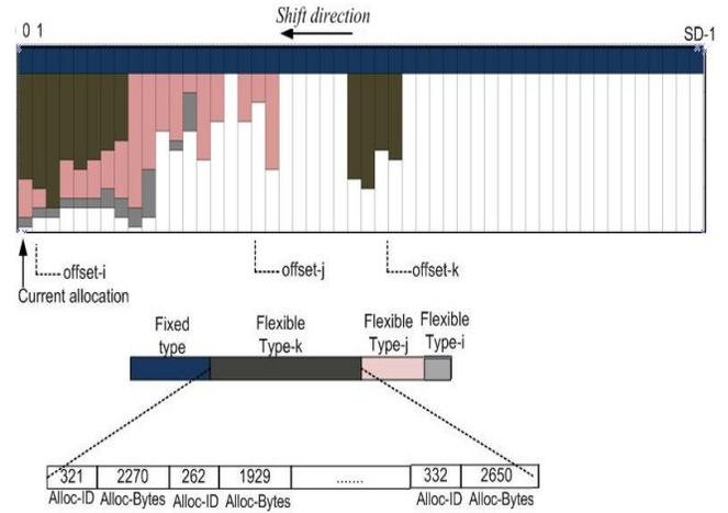
Fig. 10. Scheduling log instance for fixed type, flexible type-*i*, flexible type-*j* and flexible type-*k* Alloc-IDs in PCG-OSFI [62].
