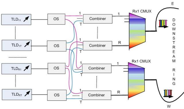
Fig. 11. OLT architecture proposed for SARDANA employing tunable laser diodes. Tunable laser diodes of the OLT operate at  $R$  optical sub-bands and are shared among the tree PONs [67].
