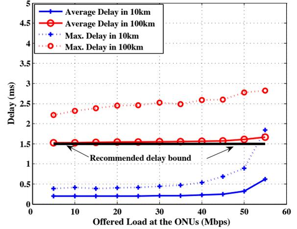
Fig. 5. Average and maximum packet delays for a case study with 10km and 100km OLT-ONU distances in an EPON.
