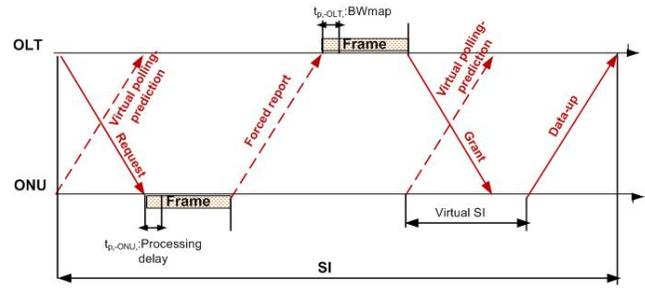
Fig. 13. Building BWmap based on status reporting in a scheduling interval [71].
