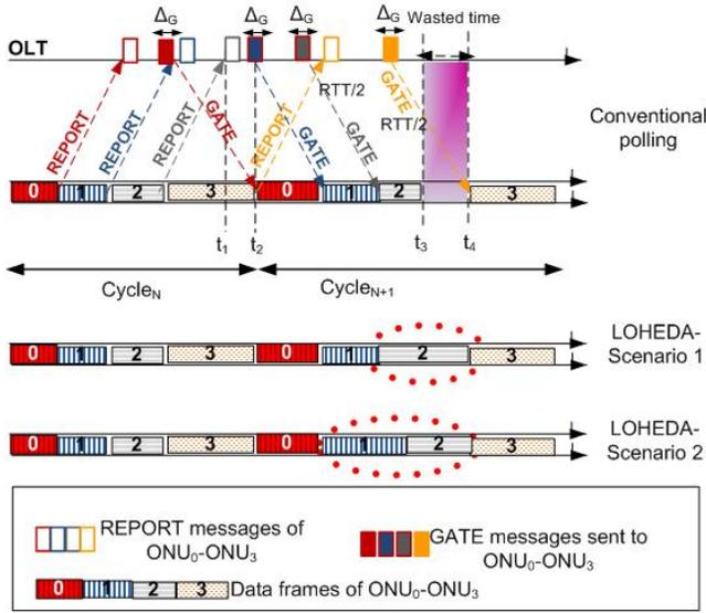
Fig. 14. Bandwidth assignment in LOHEDA. Wasted bandwidth in the regular polling mode is utilized based on the bandwidth request of ONU<sub>2</sub>. ONU<sub>2</sub> is assigned the whole wasted bandwidth (Scenario-1) or ONU<sub>1</sub> and ONU<sub>2</sub> share the wasted bandwidth (Scenario-2) [72].
