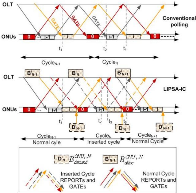
Fig. 12. Illustration of LIPSA-IC and its comparison to conventional polling [43].
