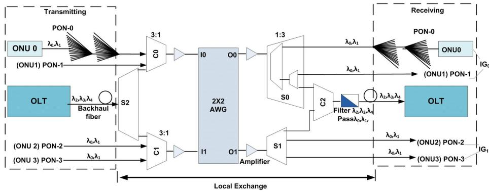
Fig. 9. SPON transmission and receiving architecture [59].
