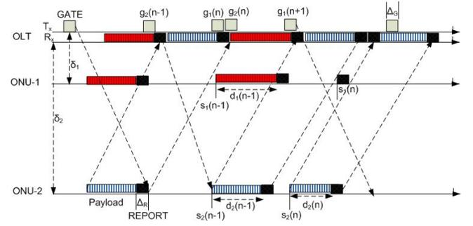
Fig. 7. Gate-Driven bandwidth allocation for two ONUs on a single wavelength [47].
