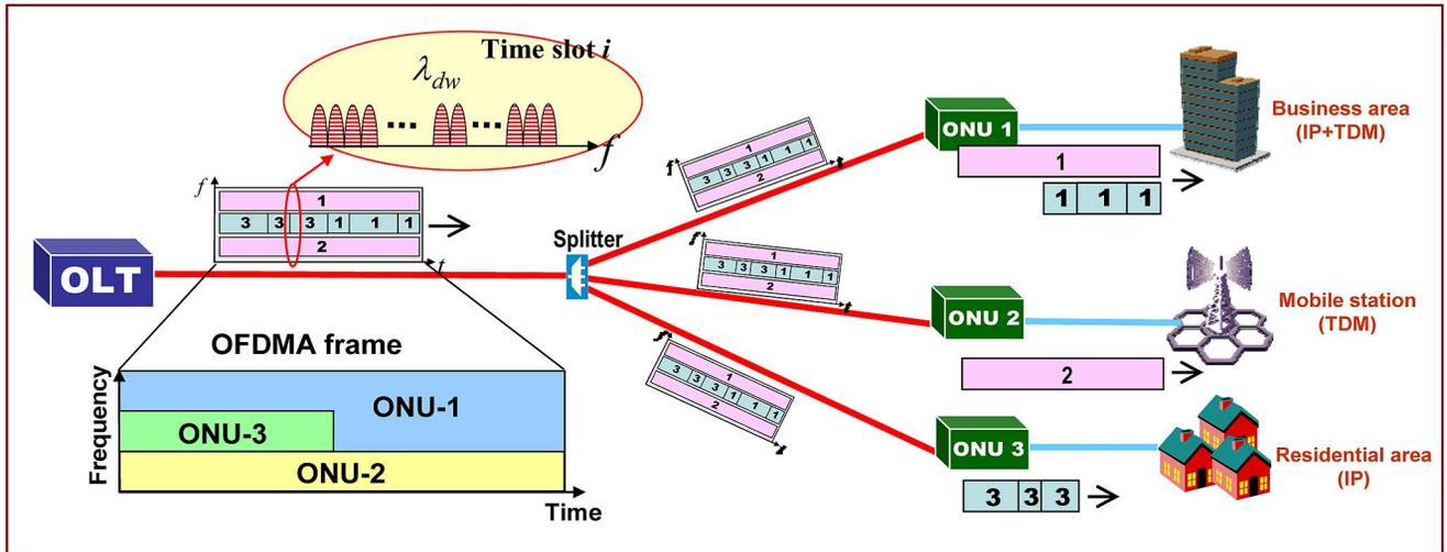
Fig. 8. Single-wavelength optical OFDMA-PON architecture for heterogeneous service delivery.
