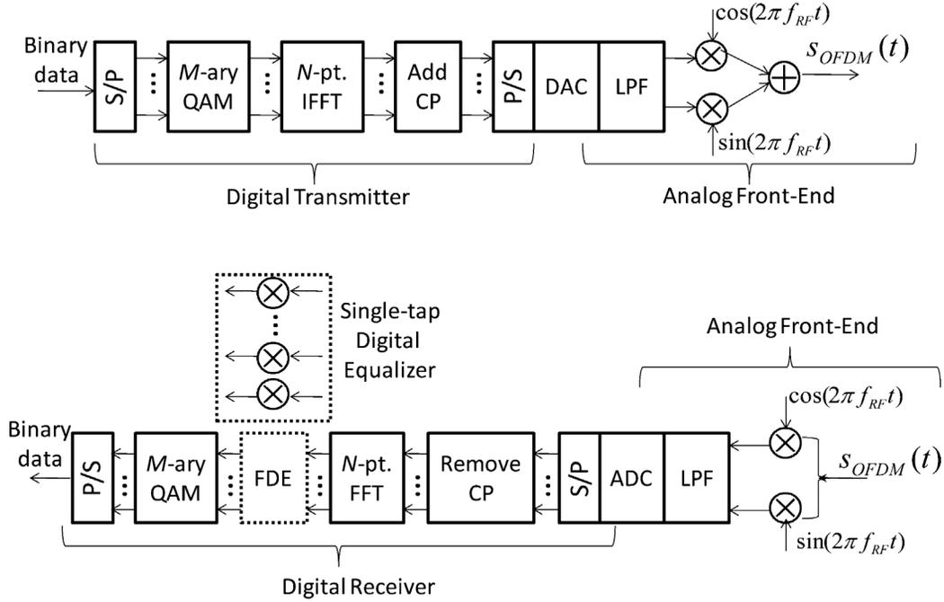
Fig. 3. Block diagram of a generic OFDM communication system.
