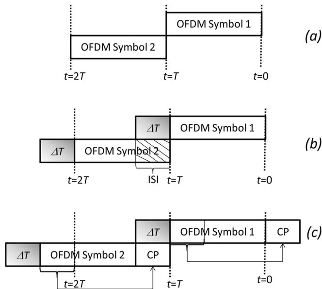
Fig. 4. OFDM symbol transmission in (a) ideal, nondispersive channel, (b) dispersive channel without CP insertion, resulting in ISI, and (c) dispersive channel with CP insertion used to eliminate ISI.
