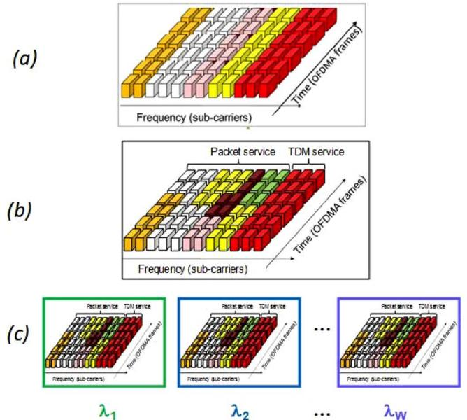
Fig. 7. Different optical OFDMA variants. (a) 1-D OFDMA with different users assigned different OFDM subcarriers. (b) 2-D OFDMA with different users assigned different OFDM subcarriers and TDM time-slots. (c) 3-D OFDMA with different users assigned different OFDM subcarriers and TDM time slots on different WDM wavelengths.
