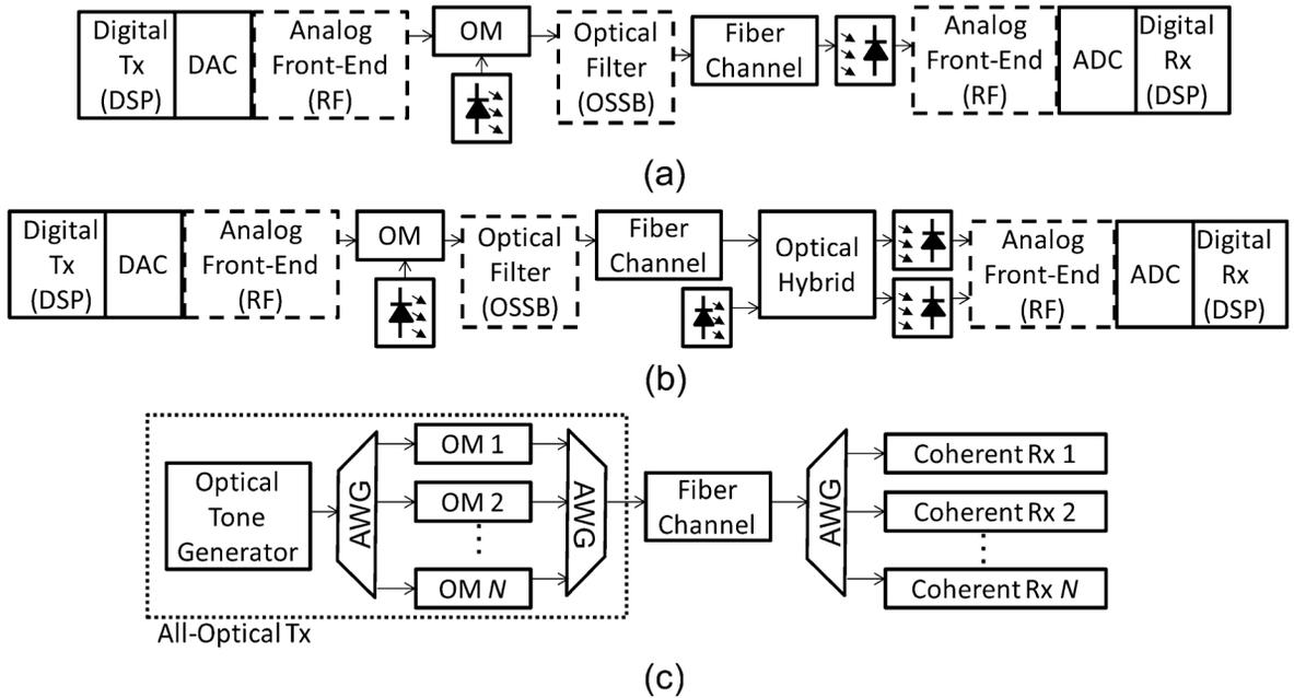
Fig. 6. Block diagram of three variants of O-OFDM. (a) O-OFDM using optical modulation (OM) with direct detection (DD). (b) CO-OFDM using optical modulation with coherent detection. (c) AO-OFDM using an optical IFFT and coherent detection. Functional blocks that may or may not be needed depending on transceiver design are denoted by dashed rectangles. (Tx= transmitter; Rx = receiver; OSSB = optical single sideband; AWG = arrayed waveguide grating).
