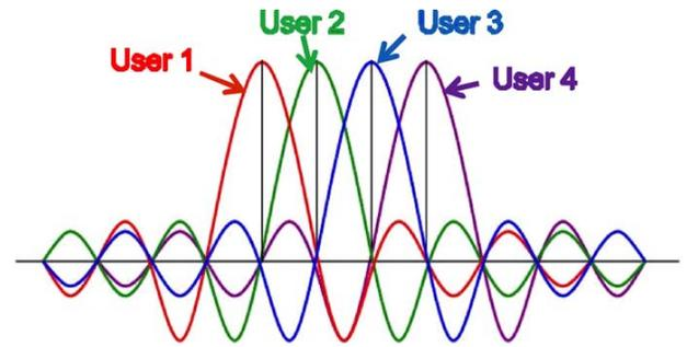
Fig. 2. OFDM(A) spectrum with four orthogonal subcarriers.
