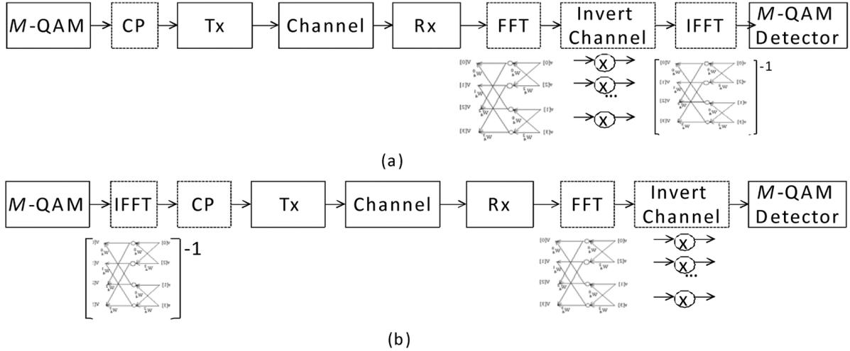
Fig. 5. System-level comparison of (a) SC-FDE and (b) OFDM communication systems.
