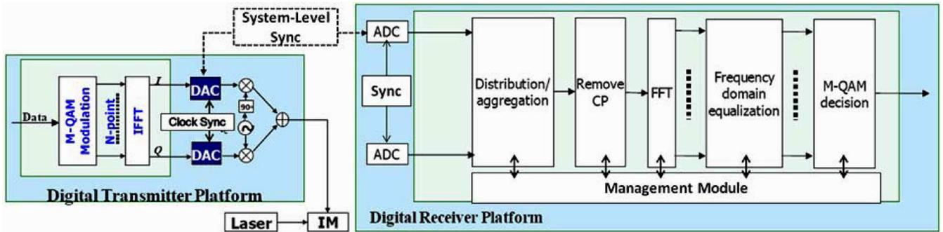
Fig. 9. Digital transmitter and receiver architectures for OFDMA-PON.
