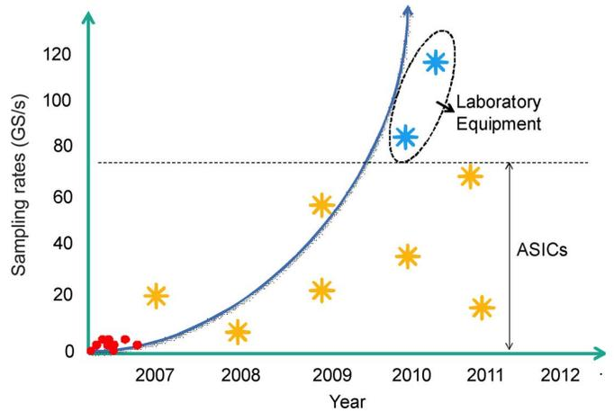
Fig. 10. Summary of recent high-speed ADC/DAC sampling rate trends.
