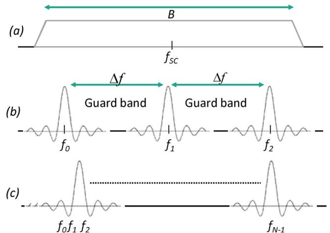
Fig. 1. Frequency-domain spectra for (a) SC, (b) FDM, and (c) OFDM signals.
