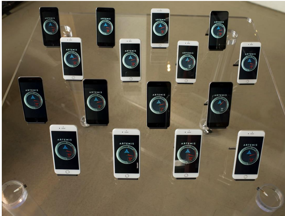
Figure 21: 1 m 2 plexiglass table with 16 iPhone 6 Plus devices
