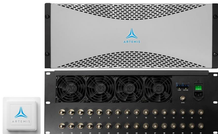
Figure 34: Artemis I Hub front/back with antenna
