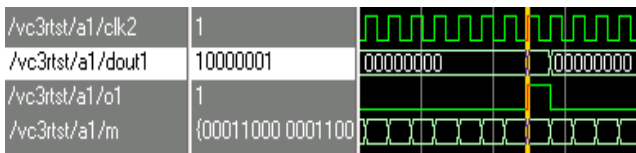
Figure 18 VC-3 buffer waveform output H4 byte for controller
