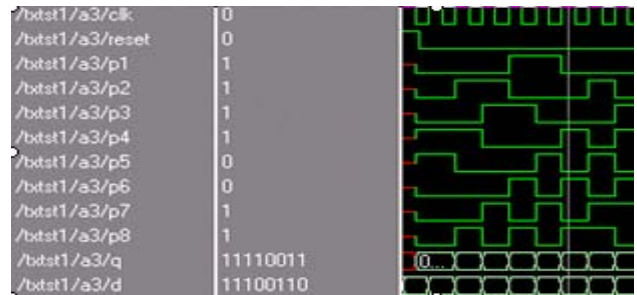
Figure 5 PRBS Generator Timing Diagram
