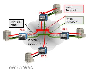
In a VPLS mesh network, each Provider Edge router must be identified and given the addresses of other PEs participating in the same VPLS. LDP sessions are then established between these PEs creating a mesh of pseudo-wires between devices. This mesh network between connected PEs enables traffic to be automatically re-routed along available backup paths, achieving much faster failover than can be supported with Spanning Tree. This creates a more reliable solution for connecting Ethernet networks
