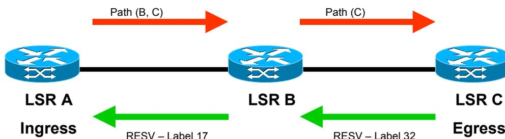
**Fig.3 RSVP LSP Setup Flow**
