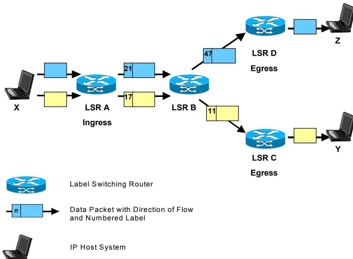
Fig.1: Two LSPs in an MPLS Network
