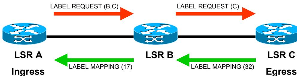
**Fig.2 CR-LDP LSP Setup Flow**
