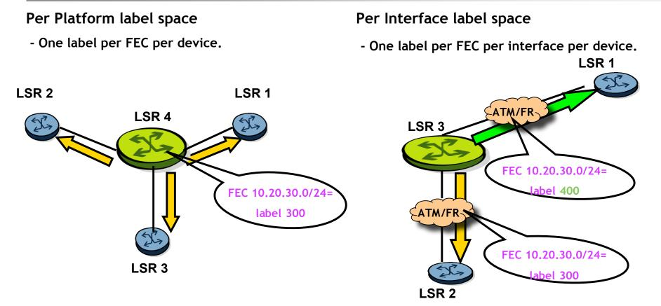
Platform wide incoming labels are used for interfaces that can share the same labels. A single label is assigned to a FEC and used across all interfaces of the same router.
