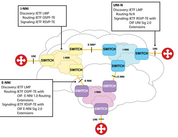
Figure 12: The Fujitsu Control Plane Approach
