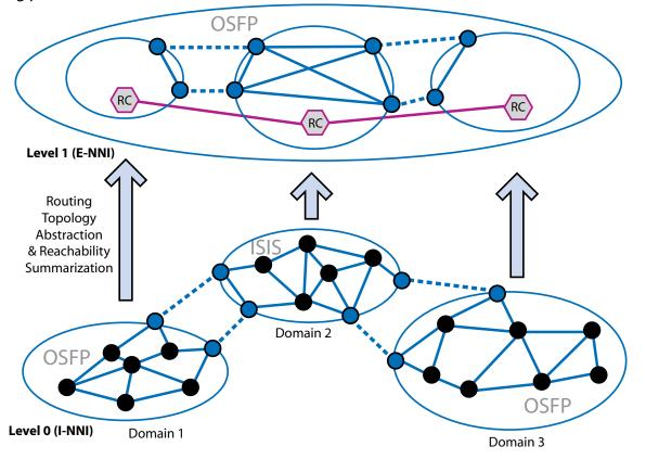
Figure 7: Single-Level Hierarchical Routing Model
