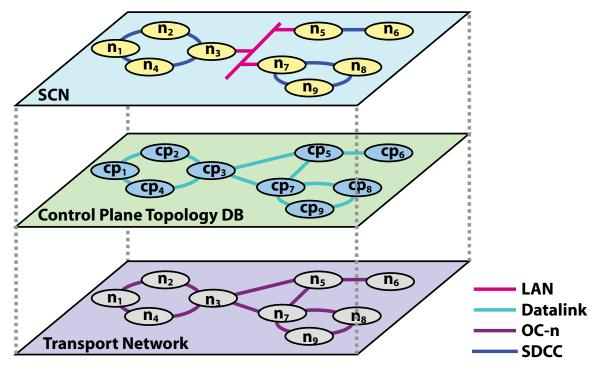
Figure 13: SCN, Control Plane, and Transport Topologies
