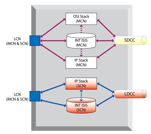
Figure 15: MCN/SCN Separated Operating Mode
