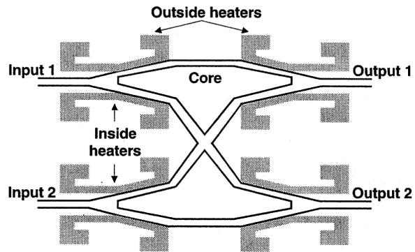
Fig. 4. Scheme of a  $2 \times 2$  digital optical switch.
