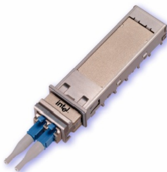
Figure 45: XFP interface physical layout
