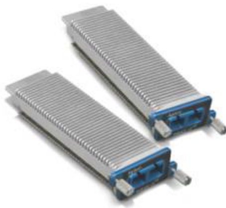
Figure 44: XENPAK interface physical layout [21]
