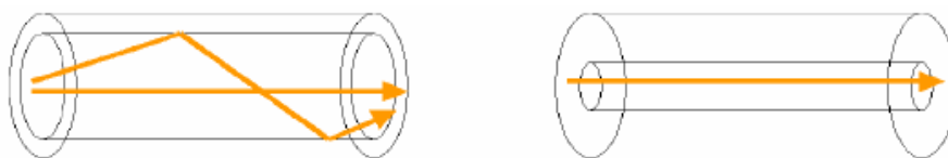
Figure 3: Multi-mode and single-mode fibres
