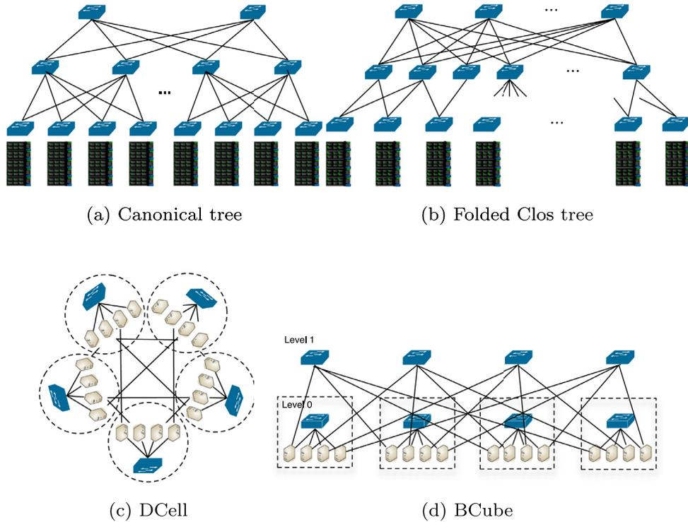
Fig. 1. Switch-centric ((a) & (b)) and server-centric ((c) & (d)) Cloud data centre topologies.
