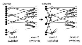
Fig. 6. Building a switch-centric DCN via Method B.
