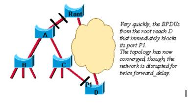
Spanning tree has been very efficient in calculating the new topology of the network. The only problem now is that twice the forward delay has to elapse before the link between the root and A eventually ends up in the forwarding state. This means 30 seconds of disruption of traffic (the entire A, B, and C part of the network is isolated) because the 8021.D algorithm lacks a feedback mechanism clearly advertising that the network has converged in a matter of seconds.
