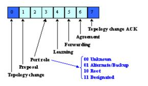
Another important change is that the RSTP BPDU is now of type 2, version 2. The implication of this is that legacy bridges must drop this new BPDU. This property makes it easy for a 802.1w bridge to detect legacy bridges connected to it.
