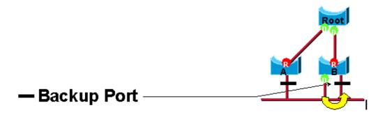
This distinction was already made internally within 802.1d. This is essentially how Cisco's UplinkFast functions. The rationale behind this is that an alternate port provides an alternate path to the root bridge and could therefore replace the root port should it fail. Of course, a backup port provides redundant connectivity to the same segment and cannot guarantee an alternate connectivity to the root bridge. It was therefore excluded from the uplink group.
