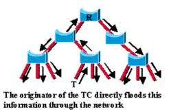
In just a few seconds (a small multiple of hello times), most of the entries in the CAM tables of the entire network (VLAN) are flushed. This approach results in potentially more temporary flooding, but on the other hand it clears potential stale information that prevents rapid connectivity restitution.
