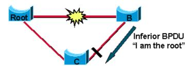
Because Bridge C still knows the root is alive and well, it immediately sends a BPDU to Bridge B containing information about the root bridge. As a result, Bridge B stops sending its own BPDUs and accepts the port leading to Bridge C as its new root port.
