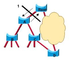
Once Switch A has blocked its non-edge designated ports, the link between Switch A and the root is put in forwarding state and we reach the situation:
