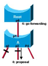
Once p0 receives that agreement, it can immediately transition to forwarding. This is Step 4 of the figure above. Notice that port p3 was left in a designated discarding state after the sync. In Step 4, that port is in the exact same situation as was port p0 during Step 1. It then starts proposing to its neighbor, attempting to quickly transition to forwarding.
