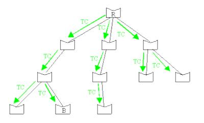
The root R sets the TC bits in its bpdus. This bpdu is relayed to the whole network.
