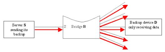
Traffic is then flooded on the whole network and will reduce the bandwidth of every single link until device D sends a frame again
