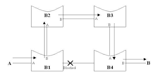
Now, let's suppose that the link between B2 and B3 fails. Communication between A and B is interrupted at least until B1 puts its port to B4 in forwarding mode (a maximum of 50 seconds with default parameters). But when A wants to send a frame to B, B1 still has an entry leading to B2 and the packet is sent to a black hole. The same applies when B wants to reach A: communication is lost for five minutes, until the entries for A and B MAC addresses age out.
