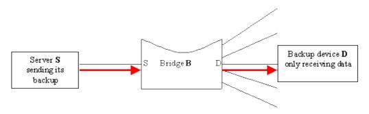
Server S is sending heavy unicast traffic to device D. Due to the nature of the protocol used, D nearly never sends any traffic. If a topology change occurs and B reduces its ageing time, entry for D will be removed from B.
