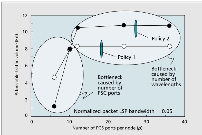
■ Figure 5. A comparison of two multilayer routing policies ( $w = 8$ ).
