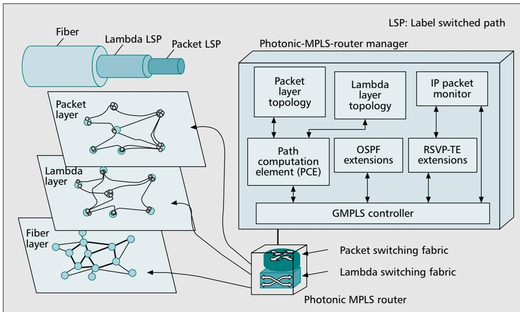
■ **Figure 1.** The structure of a photonic MPLS router with multilayer traffic engineering.
