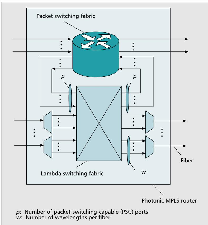
■ **Figure 2.** A node model of a photonic MPLS router.
