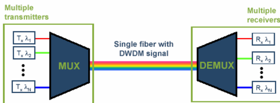
Figure: Single fiber with DWDM signal: Multiple virtual fibers
