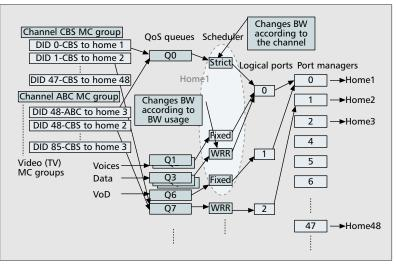
**Figure 3.** *Downstream traffic management in a line card.*
