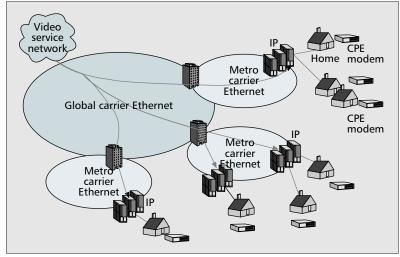
**Figure 1.** Carrier Ethernet-based IPTV network.
