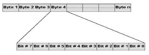
Figure 5: Bits and bytes in DENM
