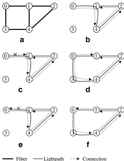
Fig. 2. Illustration of rerouting at lightpath level. Assume that each fiber has one wavelength  $\lambda_0$  and each wavelength can accommodate two connections: (a) physical topology; (b) virtual topology and connections; (c) connection request 0–1 denied before rerouting; (d) connection request 0–1 accepted after rerouting; (e) connection request 2–0 denied before rerouting; (f) connection request 2–0 accepted after rerouting.
