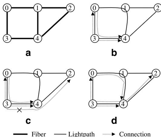
**Fig. 3.** Illustration of rerouting at connection level. Assume that each fiber has one wavelength  $\lambda_0$  and each wavelength can accommodate two connections: (a) physical topology; (b) virtual topology and connections; (c) connection request 3–2 denied before rerouting; (d) connection request 3–2 accepted after rerouting.
