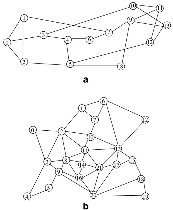
**Fig. 8.** Networks for simulation: (a) NSFNET network; (b) EUPAN network.
