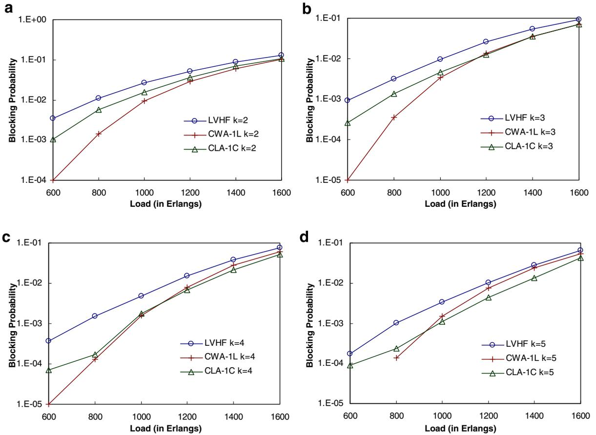
Fig. 10. Blocking performance of the rerouting algorithms in the EUPAN network: (a)  $k$  (the number of alternate paths) = 2; (b)  $k$  = 3; (c)  $k$  = 4; (d)  $k$  = 5.
