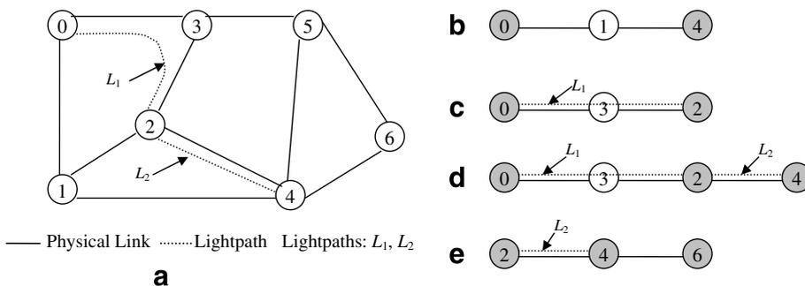
Fig. 4. Illustration of route categories: (a) the physical topology of a network and two lightpaths established on the physical topology; (b) a SN-route; (c) a SE-route; (d) an MOE-route; (e) an MNE-route.
