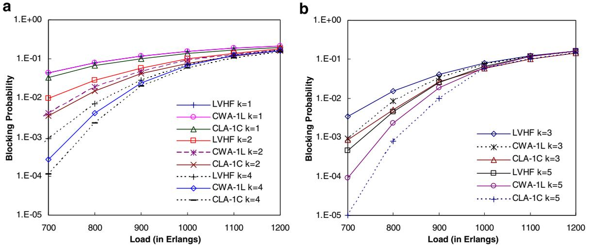
Fig. 9. Blocking performance of the rerouting algorithms in the NSF network: (a)  $k$  (the number of alternate paths) is 1, 2 and 4 respectively; (b)  $k$  is 3 and 5.
