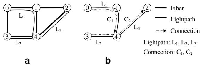
**Fig. 1.** Illustration of the two-layered routing in traffic grooming. (a) Physical topology of a five node network and three lightpaths established on the physical topology:  $L_1$  on path 0–1–4,  $L_2$  on path 3–4,  $L_3$  on path 4–2. (b) Virtual topology and two connections established on the virtual topology:  $C_1$  on lightpath  $L_1$  and  $C_2$  on path 3–4–2 using lightpaths  $L_2$  and  $L_3$ .
