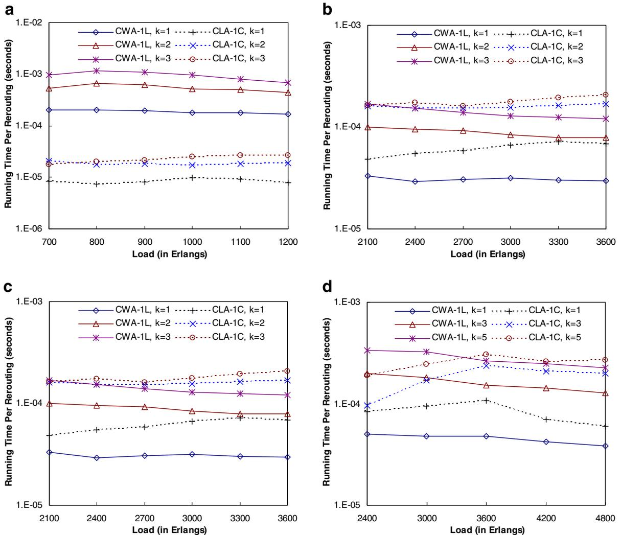
**Fig. 14.** Average running time per rerouting: (a) NSF network,  $W = 16, C = 16, G = 8$ ; (b) NSF network,  $W = 4, C = 64, G = 2$ ; (c) EUPAN network,  $W = 16, C = 16, G = 8$ ; (d) EUPAN network,  $W = 4, C = 64, G = 2$ .
