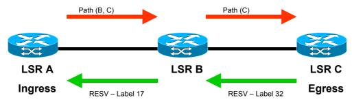
Fig.3 RSVP LSP Setup Flow
