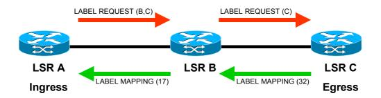
Fig.2 CR-LDP LSP Setup Flow
