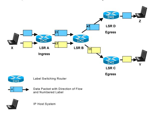
Fig.1: Two LSPs in an MPLS Network
