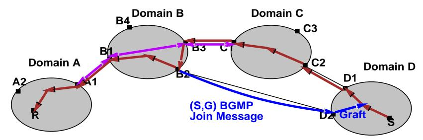
• To prevent the encapsulation and optimize the tree, B2 sends a source-specific BGMP join towards A.
