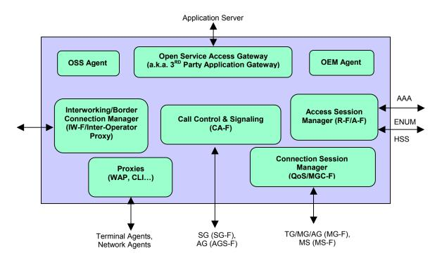
Most "Media Gateway Controller" systems today implement other functions in addition to the MGC-F. The other functions shown here (CA-F, IW-F, R-F and A-F) could be collocated on the same physical platform or distributed across different systems that together constitute a total MGC solution. Of course, for load-balancing and availability purposes, the MGC can be implemented in a cluster of systems.
