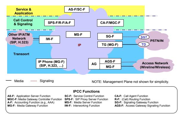
The diagram above shows 12 different functions. Understanding the autonomy of all 12 functions is an important characteristic of the IPCC Reference Architecture.
