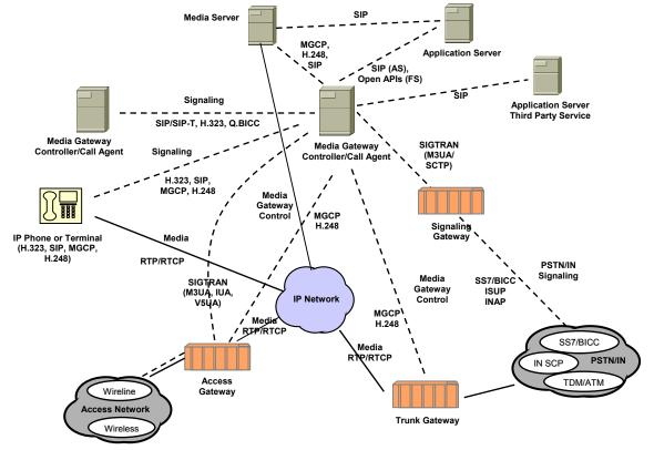
The physical entities in this example consist of the Media Gateway Controller (MGC), Applications Server (AS), Trunk Gateway (TG), Access Gateway (AG), Signaling Gateway (SG) and a Media Server (MS).
