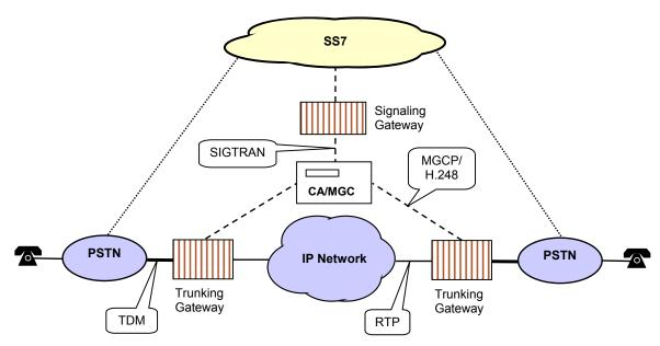
This example shows a softswitch used for tandem trunk switching, which replaces the conventional PSTN Class 4 tandem switching. The SG provides signaling transport conversion from SS7-based signaling protocols to IP SIGTRAN-based signaling protocols and transports. The TG, controlled by the MGC, provides trunking media (voice) connectivity in tandem from PSTN to IP to PSTN.
