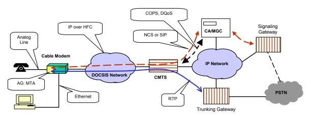
This example shows the implementation of a VoIP network using a cable access network. The cable modem at the customer premises has an embedded Multimedia Terminal Adaptor (MTA) implemented in a device called an Access Gateway (or Residential Gateway), which connects to the POTS phones and any Ethernet-based devices. An MTA can be standalone or embedded into the cable modem; a standalone MTA interfaces to the cable modem via Ethernet. The MTA terminates
