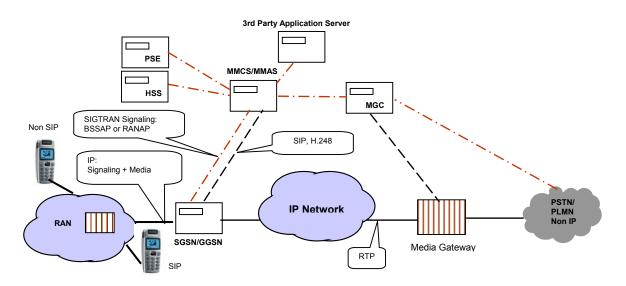
This example shows how the wireless 3G packet network connects to the PSTN or PLMN via the VoIP network. The SGSN/GGSN passes the signaling (BSSAP in GPRS or RANAP in 3G) from the radio access network (RAN) over IP to the Multimedia Server Call Server/Application Server
