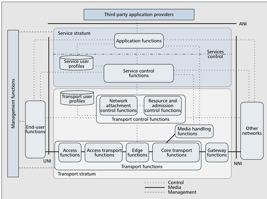
Admission control involves checking authentication based on user profiles, through the network attachment control functions. It also involves authorization based on user profiles, taking into account operator-specific policy rules and resource availability.
