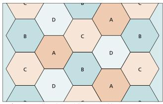
**Figure 4.** *Cells with four different sets of frequencies.*
