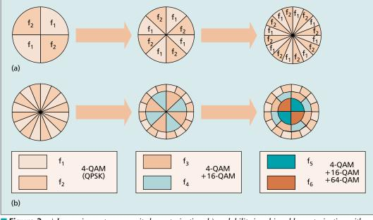
**Figure 2.** *a)* Increasing system capacity by sectorization; b) scalability is achieved by sectorization with multiple modulation schemes. Initial deployment uses 16 QPSK hubs; another eight sectors are increased by adding eight 16-QAM hubs. Further utilitzation of a full duplex channel can be achieved by adding four more 64-QAM hubs.
