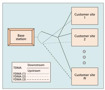
**Figure 3.** *The downstream link is multiplexed by TDMA, and FDMA is used for the upstream link.*
