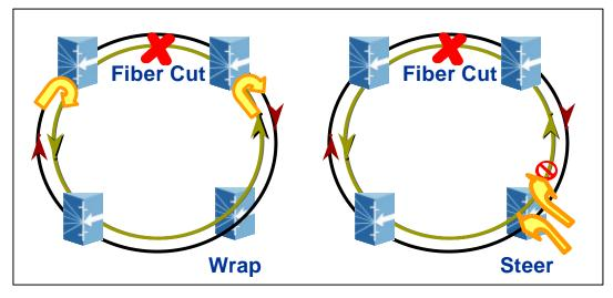
Figure 2. Wrap and Steer Protection in RPR
