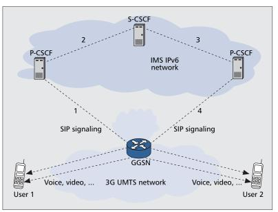
**Figure 2.** *IMS SIP signaling path (non-roaming scenario).*
