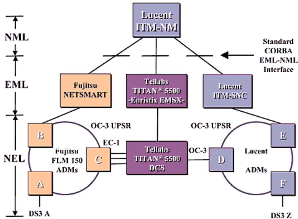
The demonstration showed point-and-click, A-to-Z provisioning on the Lucent ITM–NM network management system of a DS–3 circuit from the A point on an ADM on the Fujitsu ring through the TITAN 5500 DCS to the Z end on an ADM on the Lucent ring. This was an industry first and will lead the way to wide implementation of standards-based, easy-to-manage, multivendor networks.
